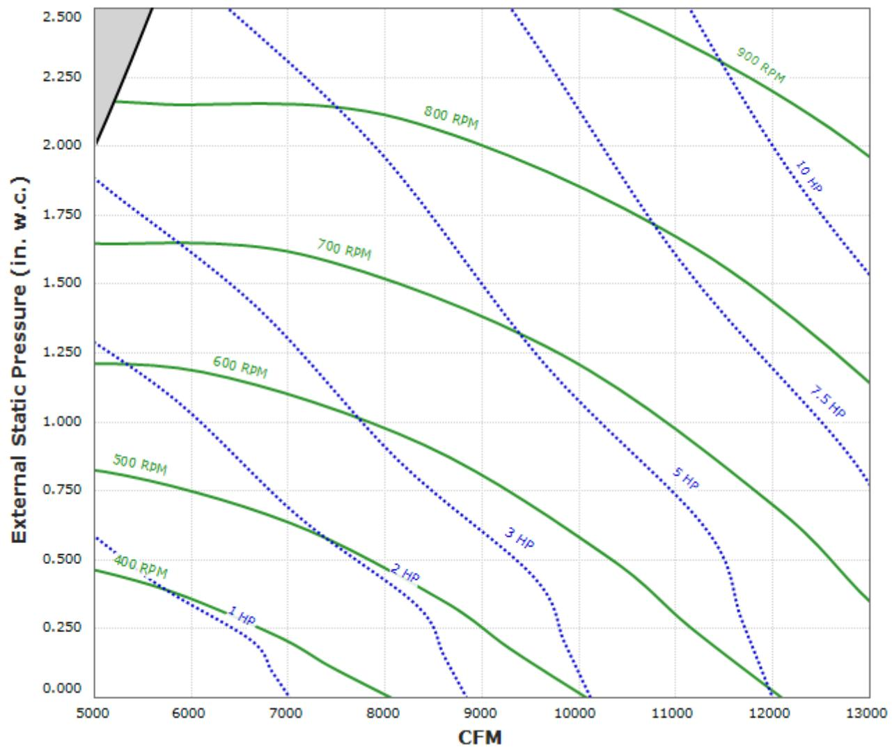
**Max Sizeable RPM = 1100 RPM. Curve shown extended beyond this point for reference only.**
