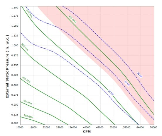
Max Sizeable RPM = 650 RPM. Curve shown extended beyond this point for reference only.
