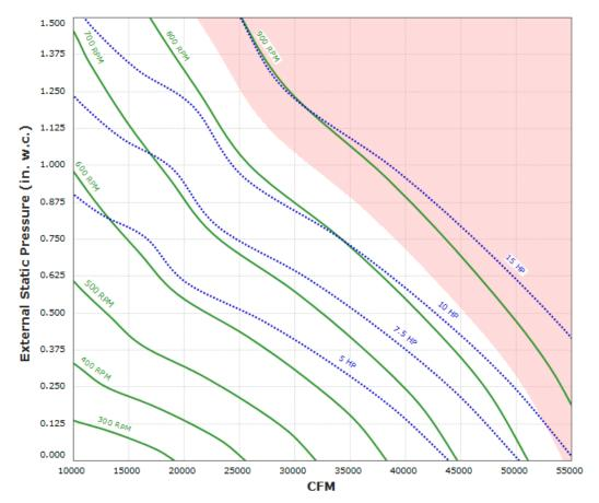
Max Sizeable RPM = 850 RPM. Curve shown extended beyond this point for reference only.
