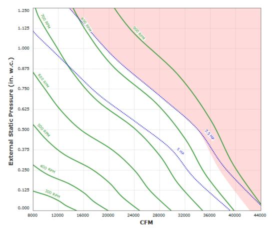
Max Sizeable RPM = 850 RPM. Curve shown extended beyond this point for reference only.
