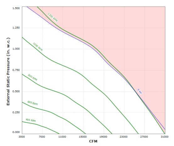
Max Sizeable RPM = 1200 RPM. Curve shown extended beyond this point for reference only.
