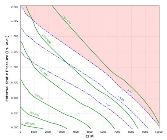
Max Sizeable RPM = 1800 RPM. Curve shown extended beyond this point for reference only.
