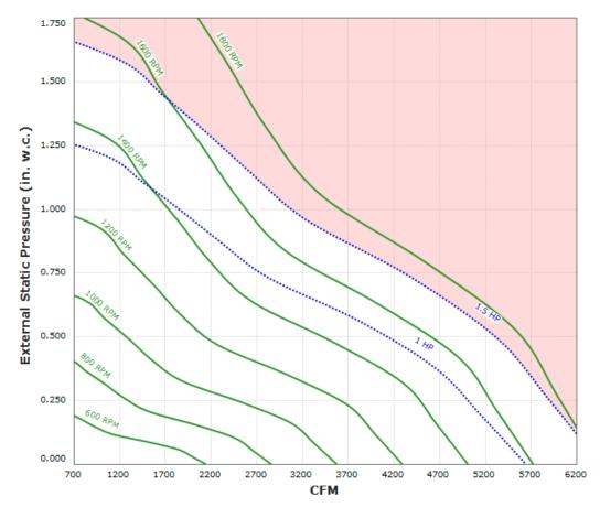
Max Sizeable RPM = 1900 RPM. Curve shown extended beyond this point for reference only.
